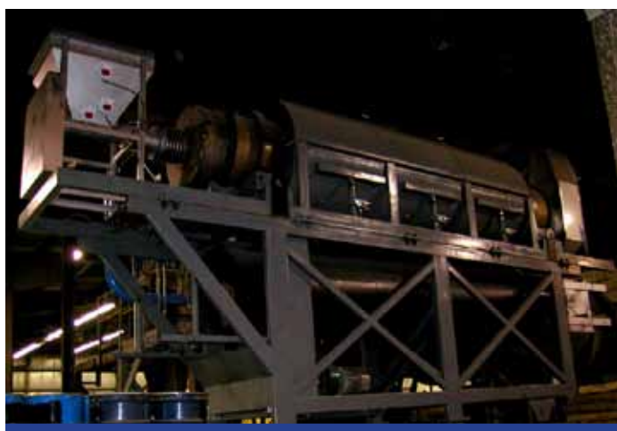
Figure 3. An in house rotary kiln eliminates up to 25% of the sulfur content and 3% of the carbon from spent catalysts. It also eliminates the need for a separate, off site pre-burn step.
