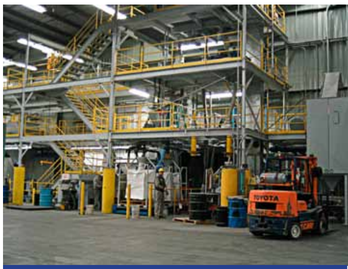
Figure 2. A continuous catalyst sampling system produces consistent, reproducible, statistically valid samples: the most important step in the recovery and refining process.
